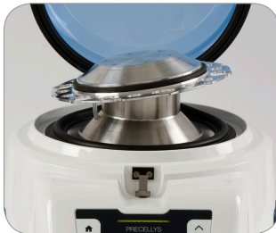
1 . Remove the indented plate
